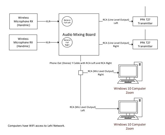
Using an old mixing board gives us some control of the audio levels present. Placing everything on the same cart and using the same power source as well as using wireless microphones eliminated any noise that sometimes occurs from ground loops. The same board can be used for two different languages by consistently treating one language as left audio and the second language as right audio.
